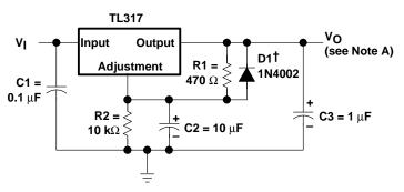
Figure 1. Adjustable Voltage Regulator
