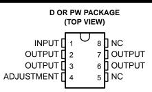
NC – No internal connection OUTPUT terminals are all internally connected.
