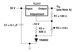
NOTE A: Output voltage is calculated from the equation:
