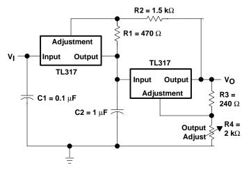
Figure 5. Tracking Preregulator Circuit
