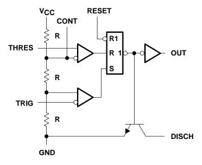
RESET can override TRIG, which can override THRES.
