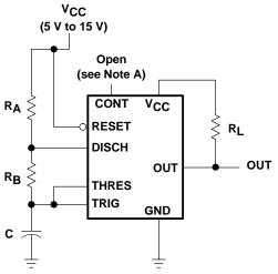
NOTE A: Bypassing the control voltage input to ground with a capacitor may improve operation. This should be evaluated for individual applications.
